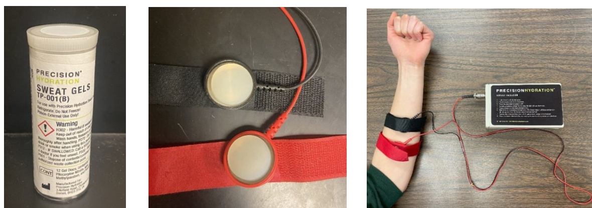
Figure 1. Precision Hydration sweat gels, pilocarpine sweat gel discs added to the electrodes, and electrodes attached to the sweat inducer and the forearm of the subject.
